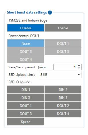
When the Iridium edge device is connected *Power control DOUT* configures DOUT pin which can control Iridium Edge ON/OFF pin. Configure if DOUT pin is connected. Respective power control DOUT to which the Iridium device's *PIN6* is connected must be selected.
