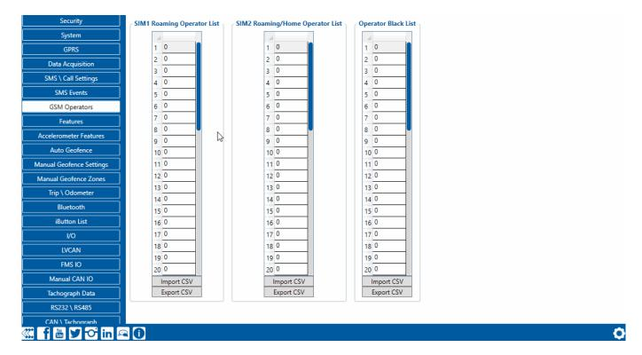
If roaming operator list is left empty, FMB640 will automatically detect home operator. If home operator is written to the roaming operator list, it will still be detected as home operator. Any operator not in the roaming operator list (except the home operator) will be recognized as unknown operator and FMB640 will work in Unknown mode (make sure it is configured to allow data sending – GPRS context is enabled).
