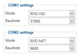
The difference between *RFID HID Mode* and *RFID MF7 Mode* is that in *RFID HID Mode* FMB640 understands RFID messages that are in hexadecimal format and *RFID MF7 Mode* interpretes messages that are in decimal format. The type of RFID message sent to FMB640 depends on the RFID reader. For example, *RFID HID* mode message looks like "\$aa\$02\$03\$04\$17\$89\$00\$01" while *MF7 mode* message is of following format: "1213141519".
