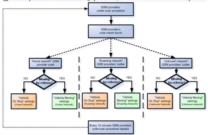
Operator search is performed every 15 minutes. Depending on current GSM operator Home, Roaming or Unknown mode can be changed faster than every 15 minutes. This process is separate
