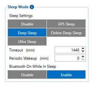
Note: In case when during scan after wakeup no BLE devices will be found FMB will be active for configured scan duration time in Bluetooth 4.0 tab. After that timeout FMB will go to sleep state.
