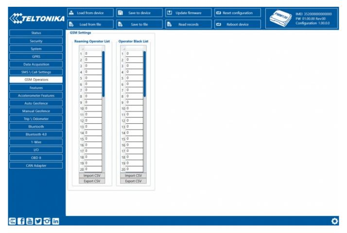
If roaming operator list is left empty, FMB1YX will automatically detect home operator. If home operator is written to the roaming operator list, it will still be detected as home operator. Any operator not in the roaming operator list (except the home operator) will be recognized as unknown operator and FMB1YX will work in Unknown mode (make sure it is configured to allow data sending – GPRS context is enabled).
