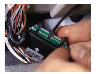
4. Connect CAN adapter **positive** and **ground** wires to the vehicle power supply lines or near FMM125 power wires.
