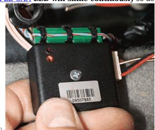
**Press the switch shortly** and wait for the LED to start blinking **every one second**.
