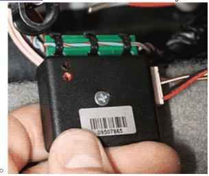
**Press the switch shortly** and wait for the LED to start blinking **every one second**.
