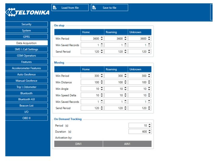
Min Saved Records defines minimum number of coordinates and I/O data that should be transferred within a single connection to the server. If FMU1YX does not have enough coordinates to send to the server, it will check again after a time interval defined in Send Period field.
