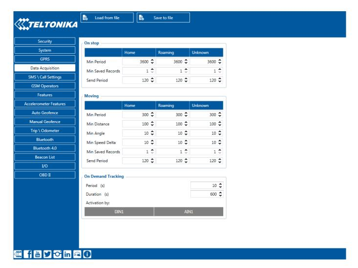
There are three available options for the activation source of tracking on demand - DIN/AIN or both (devices that support multiple DINs/AINs allow choosing which DINs/AINs to use). Note that, these inputs will work as buttons, rather than switches, and are used to trigger the functionality, the duration of tracking on demand will not be extended if the activation source status is high for a period of time.
