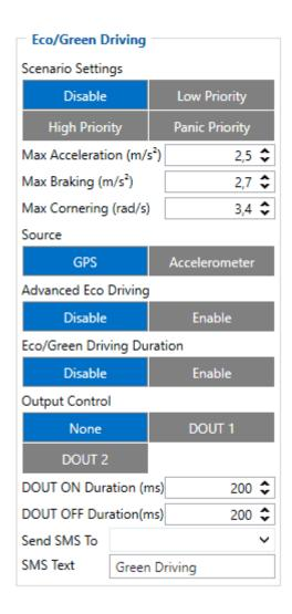
When vehicle parameters exceed the values of Max Acceleration, Max Braking or Max Cornering parameters, the scenario is activated: a record is generated, and the digital output status is changed to 1 when configured. You can configure all three parameters in  $m/s^2$  units. The scenario is activated until the current Acceleration, Braking, or Cornering value decreases below the set parameter value. Parameters used with Eco/Green Driving functionality are given in a table below.
