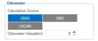
Calculation Source allows to choose Odometer calculation source between GNSS, LVCAN or OBD. Odometer Value sets the starting total odometer value.
