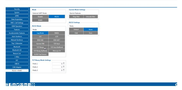
TCP Binary has a setting Prefix. It is possible to set Prefix 1, Prefix 2, or Prefix 3. These prefixes can be used separately or in unison. To configure this setting a value from 0 to 255 in decimal has to be entered. The device will convert this value to HEX and compare the 1st, 2nd, or 3rd byte from incoming data. If the values do not match, the device will not accept incoming data.
