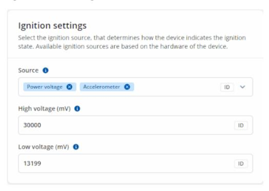
Ignition source will be used to determine the ignition status of the vehicle.
