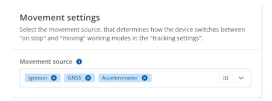
Movement source will be used to determine when a vehicle is on stop or moving. Possible movement sources:
