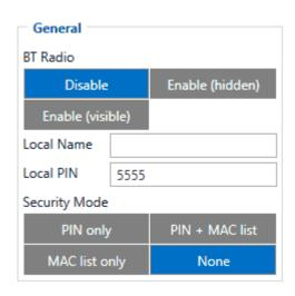
General functionality configures Bluetooth to work in slave mode. This mode allows any external device to connect to FMB1YX.
