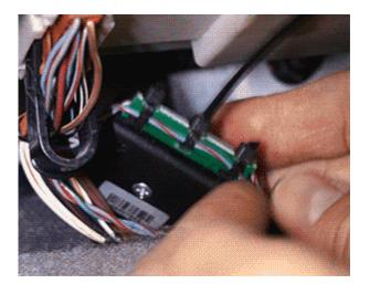
4. Connect CAN adapter **positive** and **ground** wires to the vehicle power supply lines or near FMC130 power wires.
