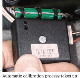
Automatic calibration process takes up to 10 seconds depending on the vehicle model. Device is calibrated properly then the LED is blinking **every 2 seconds**.
